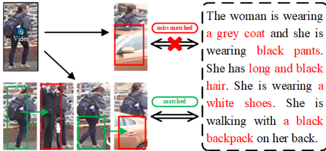
Figure 2: The occlusion problem in a single video frame will cause the failure of the matching between text and video, but multiple video frames can solve the occlusion problem.
